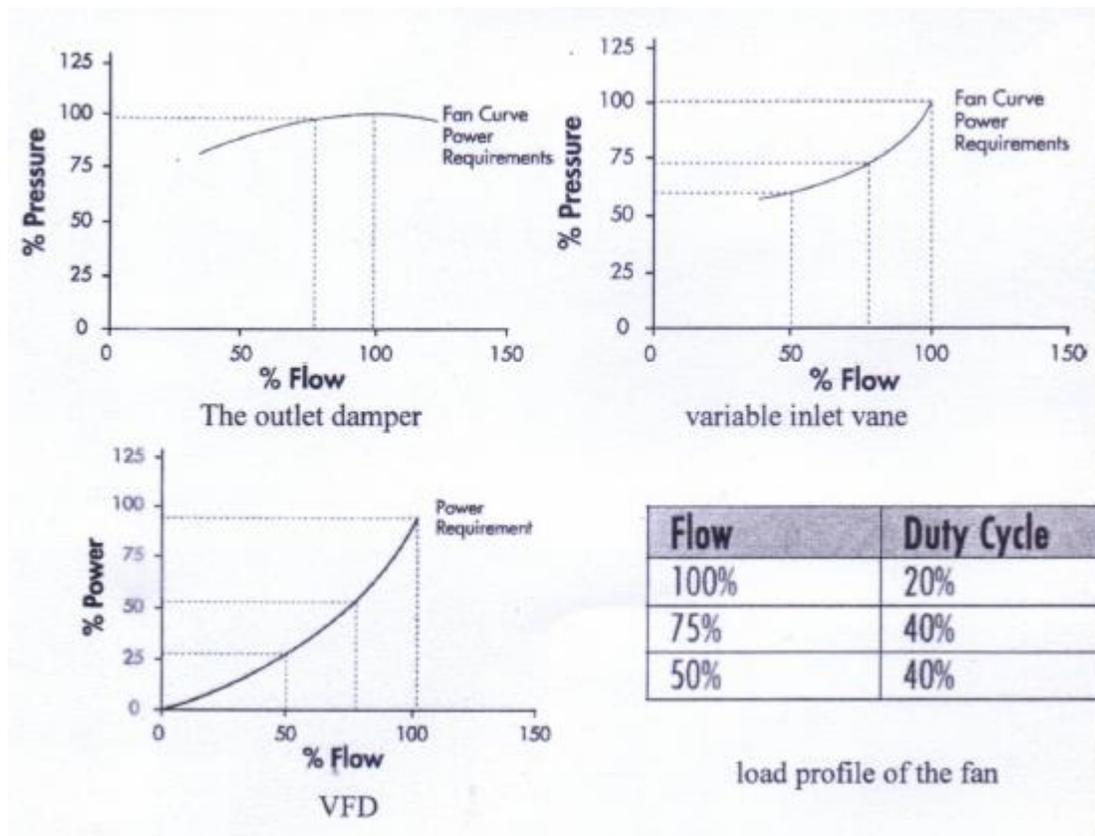
2. A plant's ventilation system used 10, 40-hp motors on a 24/7 basis except for a 2-week shut down in a year. The current motors are 85% efficient at rated/full load. Management is considering updating the motors with 93%-efficiency motors at \$2000 each. They pay 6 cents/kWh for electricity. Assume load has been closed to rated/full load. What is the payback period and ROI? 10
